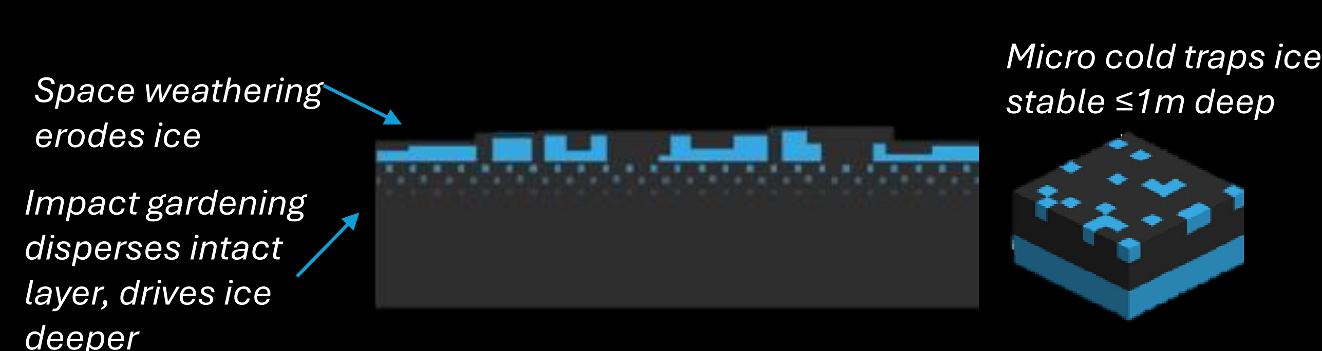
Figure 3*: TTII contains volatiles ≤1m below the surface, instruments specializing in subsurface measurements such as ground-penetrating radar and drilling are required.
